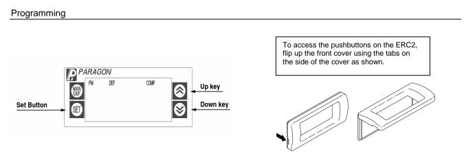
The ERC 2 control initially powers up displaying 12:00 AM otherwise it will show the last configured selection (time or temperature). If a power outage occurs during normal operation, the control will maintain the correct time-of-day using a capacitor (batteries are not required). The time will be maintained for up to 100 hours when the capacitor is fully charged.
